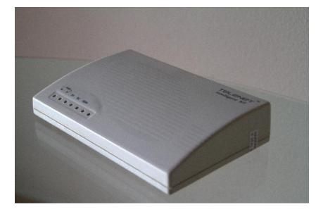
The ISDN TA with built in NT is an ISDN network Terminator with 2 a/b (POTS) ports with serial and USB built in data ports. The data port provides a high speed solution for internet access, File transfers, Remote Access services etc. Support for advanced communication software is provided via CAPI 2.0 drivers.
