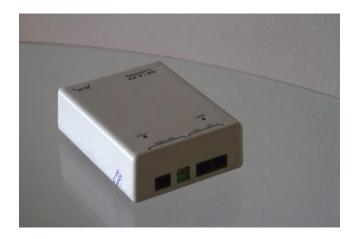
Telenet's ISDN Network Termination for basic rate access is the main gate to the world of ISDN. It enables subscribers to use services such as high-speed transmission of data, text and video signals in digital format over an access line in addition to voice transmission. It is a link between the subscriber line (U Interface) and the user Interface to the network (S/T interface). A maximum of 8 terminal units can be connected to the S/T interface.
